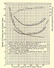
Fig. 266.—Characteristic performance graphs of the uniflow engine.\*
